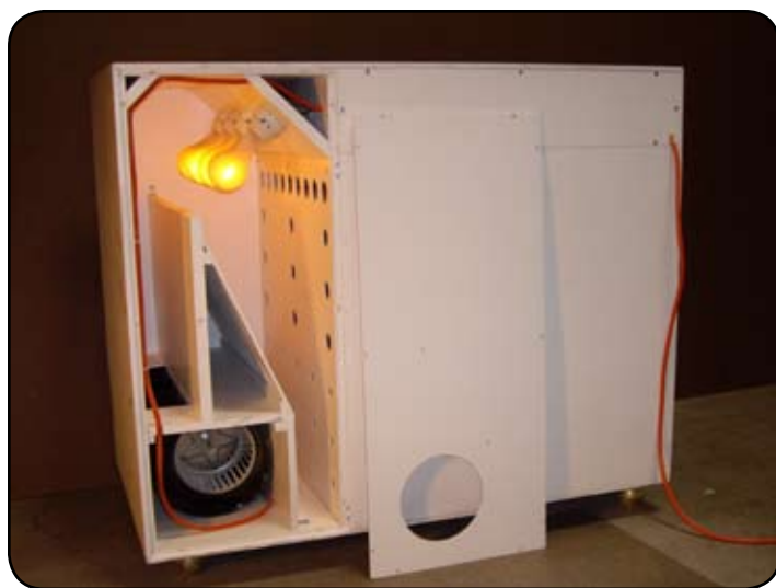
Rear view of the dehydrator, with the airflow chamber uncovered. Photo by Dan Long
