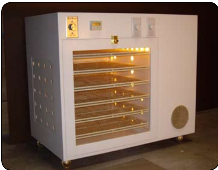
Front view of the dehydrator, with air outlet holes on the left and intake filter on the bottom right. Photo by Dan Long
